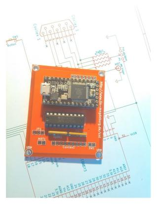
Via USB cable the Teensy Box is connected with your stimulus PC / Laptop and will be recognized as USB HID keyboard without driver installation (Windows, Mac OS, Linux). We use a Teensy board programmed using a simple teensyduino sketch. All variants listen for input pulses from the MR scanner and for pulses from the response buttons. The input is converted to keyboard events:
