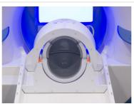
Siemens (Nova Medical) TxRx 24-Channel Head Coil (no visual stimulation)
